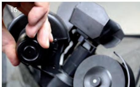
The plastic disc can now be removed from the motor shaft. (Fig. 17.a, b,) Remove the plastic disc from the projection wheel (which is held together by three screws) and replace it with a new one.
