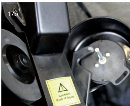
Slide the new wheel onto the end of the axis and tighten the screw. Then adjust the correct distance of the wheels with the help of the adjustable tube as described above.
