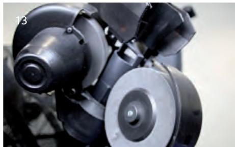
**Please note:** The correct distance between the wheels should be 36-37 mm.
