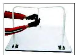
Attach the steel strip using the knob at both ends & screw the knob.
